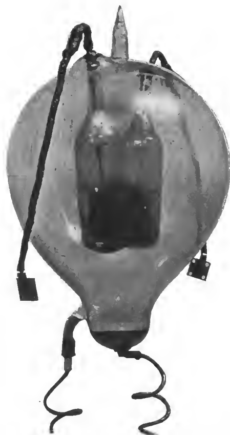
GLASS BULB OF HEWITT CONVERTER, SHOWING TERMINALS AND MERCURY POCKETS
